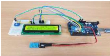
Fig. 11: DHT11 Sensor Measuring Temperature and Humidity.
