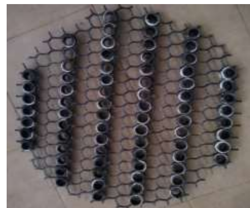
Fig. 1 (b) Top view of Geogrid with PVC pipes (3D geogrid)
