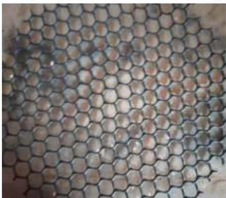
Fig. 1 (a) Top view of Geogrid (2D geogrid)
