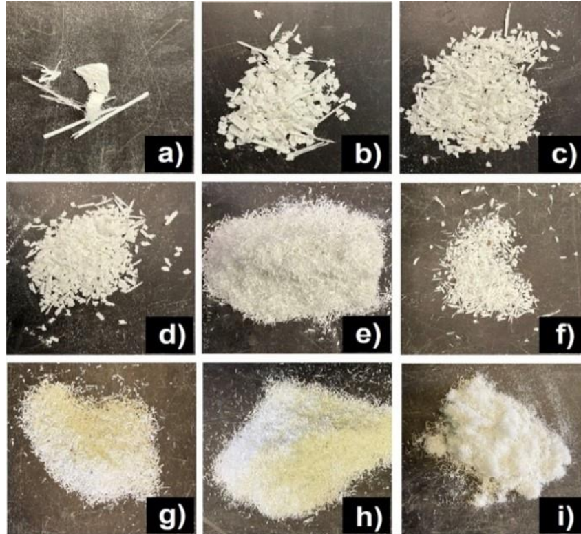
Fig. 4 Remaining fractions of crushed GFRP waste on the sieves, a) 5.6 mm, b) 4.0 mm, c) 3.2 mm, d) 2.8 mm, e) 2.0 mm, f) 1.4 mm, g) 1.0 mm, h) 0.50 mm, i) <0.5 mm
