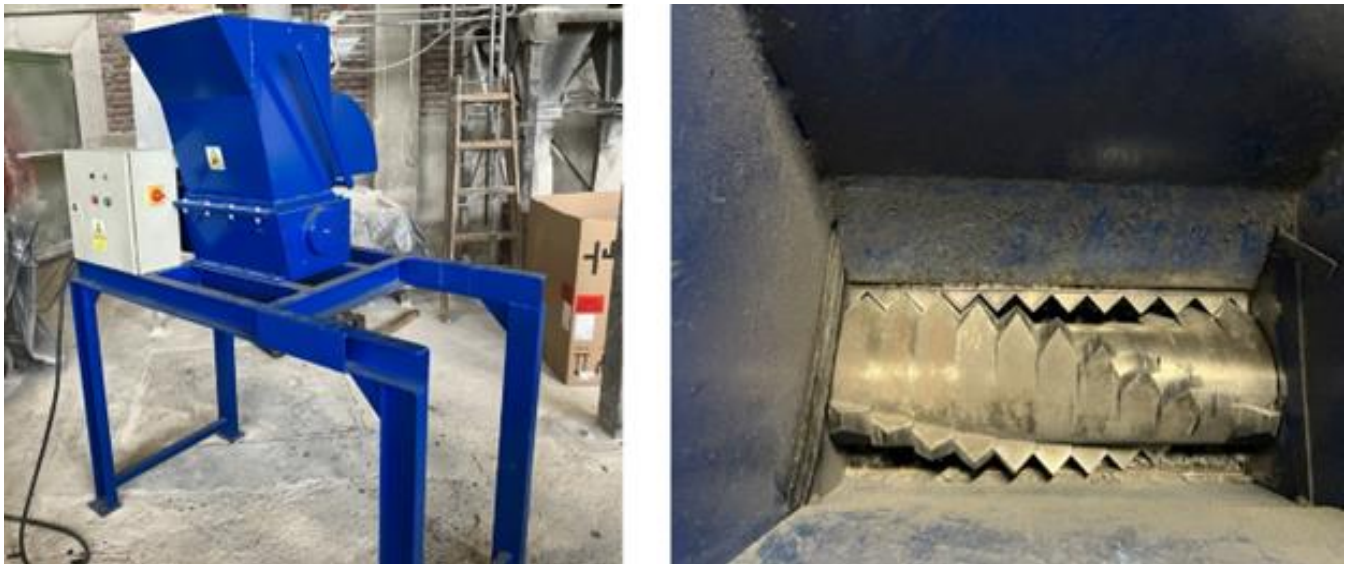
Fig. 2 Single-shaft knife crusher (on the left), crushing element (on the right)
