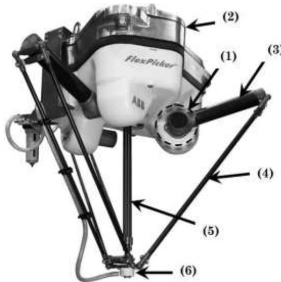
Fig.1. The General Mechanical Structure of delta robot: 1) Three Actuators. 2) Base plate 3) Upper robot arm 4) Lower robot arm (Forearm) 5) Rotation arm (optional, 4-DOF) 6) Travelling plate, TCP
