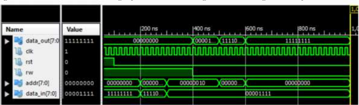
Fig. 4: Simulation Waveform single port RAM with single read and single write operations
