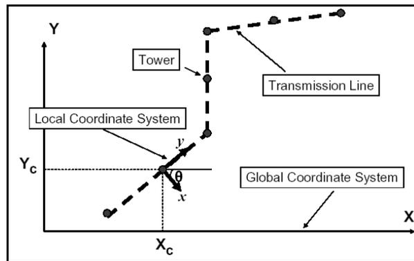
Figure 5 Coordinate Systems used in defining a transmission line
