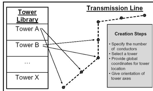
**Figure 6** Construction of a transmission line section
