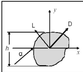
Figure 9 Aerodynamic forces acting on a member with arbitrary cross-section
