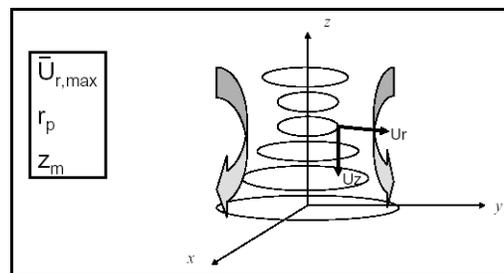
**Figure 7** OBV downburst profile in a local coordinate system
