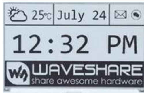
Figure 20. E-paper display for smart bags that can be changed for context and purpose
