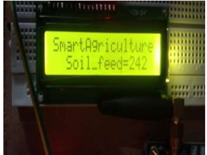
Sensor value when soil is wet
