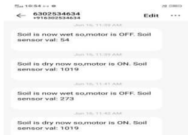
Soil is dry so motor is on. Sensor value is given.
