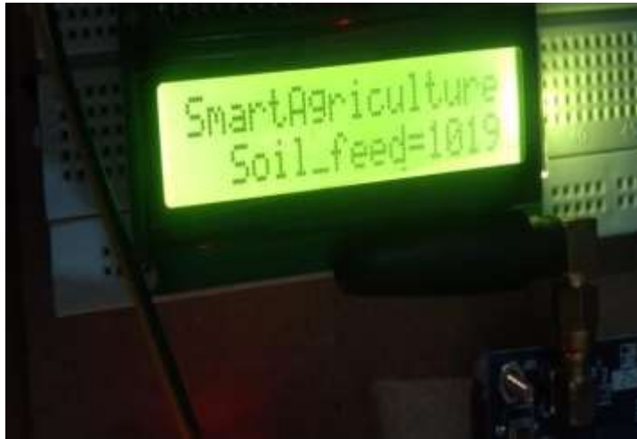
Soil is dry so motor is on. Sensor value is given.
