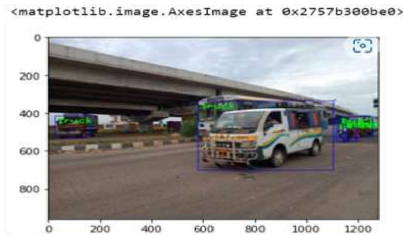
Fig.9 Results of object detection when there are vehicles
