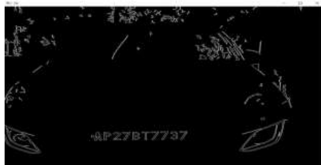
Figure-8(a): Detection of Characters on Number Plate
