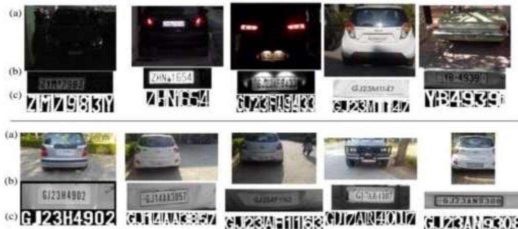
Figure-10: Output for License Plate in Different Lighting Conditions
